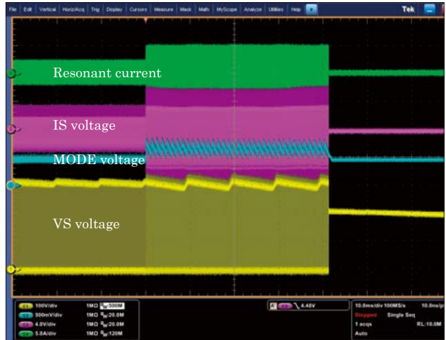
Fig.9 Waveform during over-current protection operation
