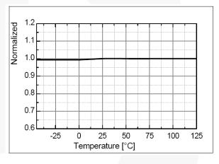
Figure 13. Current-Sense Input Threshold Voltage Limit (V<sub>CS</sub>) vs. T<sub>A</sub>
