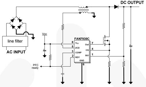
Figure 1. Typical Boost PFC Application
