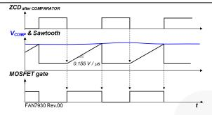
Figure 33. Turn-On Time Determination
