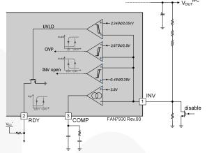
Figure 23. Circuit Around INV Pin
