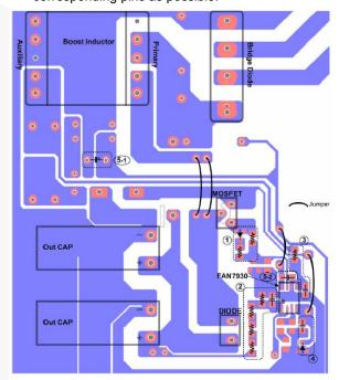
Figure 44. Recommended PCB Layout
