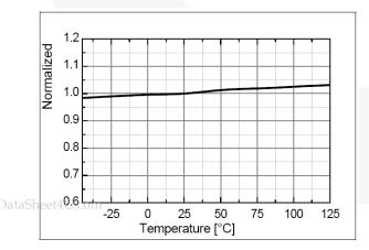
Figure 14. Input High Clamp Voltage (VCLAMPH) vs. TA
