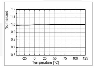
Figure 21. OVP Threshold Voltage (V<sub>OVP</sub>) vs. T<sub>A</sub>
