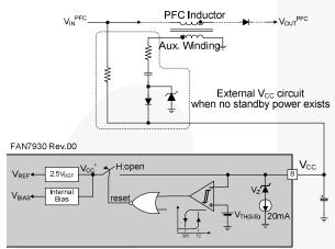
Figure 22. Startup Circuit
