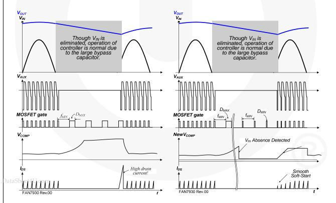
Figure 42. Operation without VIN Absent Circuit
