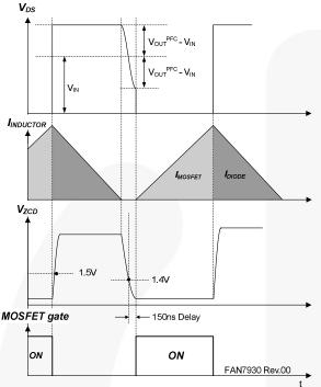
Figure 29. Auxiliary Voltage Threshold
