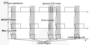
Figure 31. Maximum Switching Frequency
