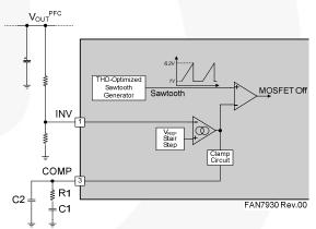
Figure 32. Control Circuit
