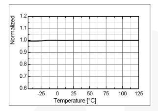
Figure 10. Zero Duty Cycle Output Voltage ( $V_{\text{EAZ}}$ ) vs.  $T_{\text{A}}$
