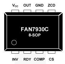
Figure 3. Pin Configuration (Top View)
