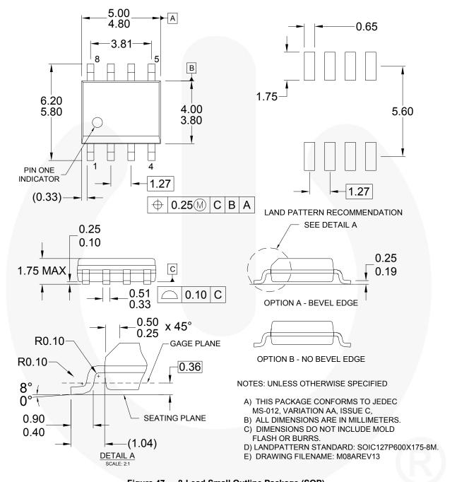
Figure 47. 8-Lead Small Outline Package (SOP)
