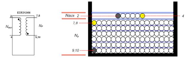
Figure 46. Transformer Schematic Diagram
