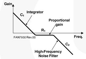
Figure 34. Compensators Gain Curve
