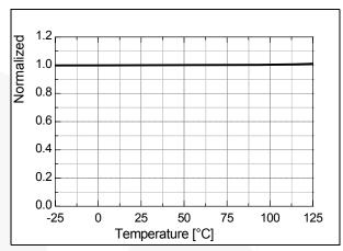
Figure 5. UVLO Start Threshold Voltage (V<sub>START</sub>) vs. T<sub>A</sub>
