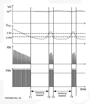
Figure 22. Waveforms of Burst Operation
