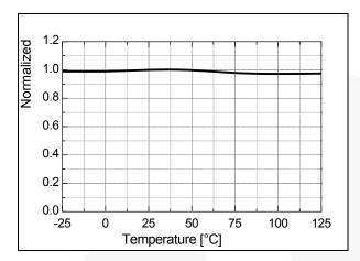
Figure 10. Over-Voltage Protection (V<sub>OVP</sub>) vs. T<sub>A</sub>
