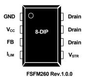
Figure 3. Pin Configuration (Top View)
