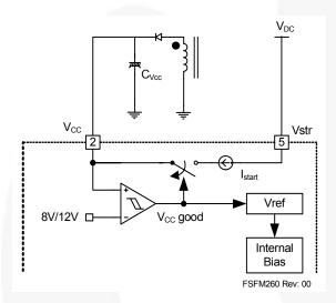
Figure 16. Internal Startup Circuit
