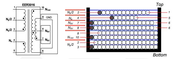
Figure 25. Transformer Schematic Diagram
