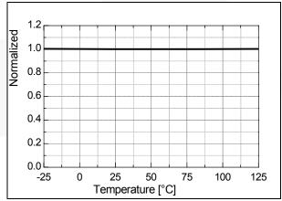
Figure 9. Maximum Duty Cycle ( $D_{MAX}$ ) vs.  $T_A$
