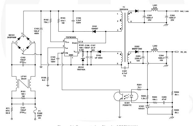
Figure 24. Demonstation Circuit of FSFM300N
