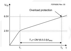
Figure 20. Overload Protection
