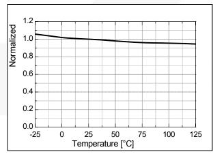
Figure 15. Peak Current Limit (I<sub>LIMIT</sub>) vs. T<sub>A</sub>
