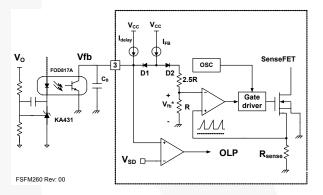
Figure 17. Pulse Width Modulation (PWM) Circuit
