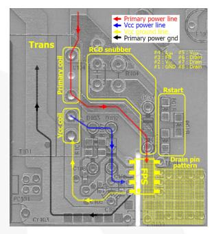
Figure 23. Recommended PCB Layout
