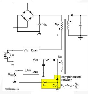
Figure 18. Constant Power Limit Circuit
