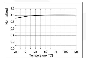
Figure 8. Switching Frequency (f<sub>OSC</sub>) vs. T<sub>A</sub>
