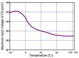
Fig. 4 Maximum Input Voltage of CS pin vs. Temperature
