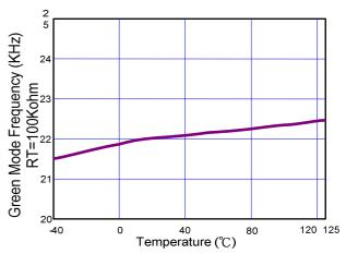
Fig. 6 Green Mode Frequency vs. Temperature
