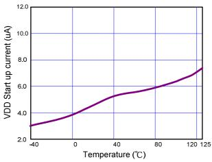
Fig. 1 VDD Start up current vs. Temperature
