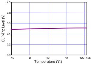
Fig. 3 OLP Trip Level vs. Temperature
