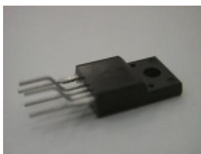
1. Drain 2. GND 3. V<sub>CC</sub> 4. FB 5. Sync**FEATURES**
