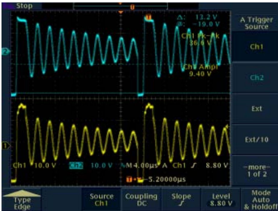
pic.3 secondary winding output and gate voltage of MOSFET waveform at no load condition .
