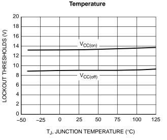
Figure 22. Supply Voltage Undervoltage Lockout Thresholds vs. Temperature
