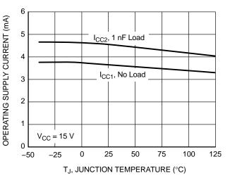
Figure 24. Operating Supply Current vs.
