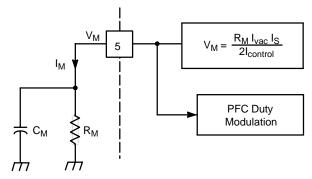
Figure 29. External Connection on the Multiplier Voltage Pin
