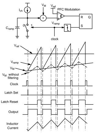
Figure 27. PFC Duty Modulation and Timing Diagram
