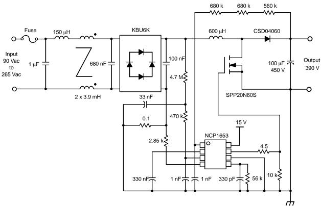
Figure 42. 300 W 100 kHz Power Factor Correction Circuit
