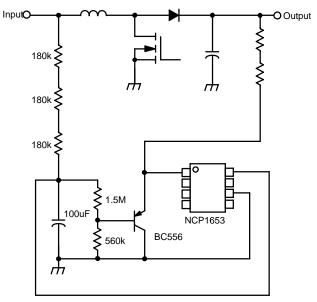
Figure 41. Recommended Startup Biasing Scheme
