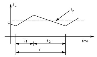
Figure 26. Inductor Current in CCM
