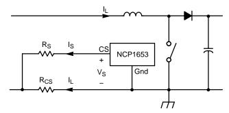
Figure 36. Current Sensing
