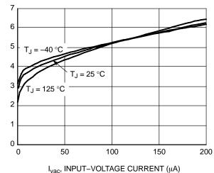
Figure 18. In Pin Voltage vs. Input-Voltage Current
