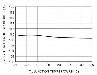
Figure 12. Overvoltage Protection Ratio vs. Temperature
