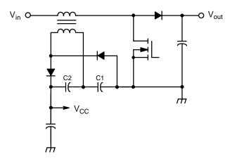
Figure 40. Self-biasing Scheme in Constant Output Voltage Mode
