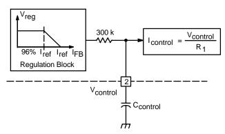
Figure 30. V<sub>control</sub> Low-Pass Filtering
