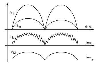
Figure 28. Multiplier Voltage Timing Diagram
