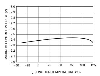
Figure 9. Maximum Control Voltage vs. Temperature
