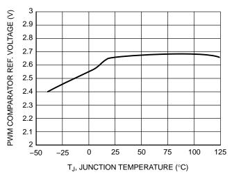
Figure 19. PWM Comparator Reference Voltage vs. Temperature
