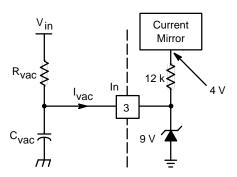
Figure 37. Input Voltage Sensing
