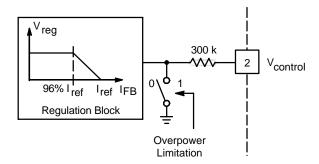
Figure 38. Overpower Limitation Reduces V<sub>control</sub>
