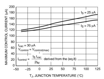
Figure 20. Maximum Control Current vs.
