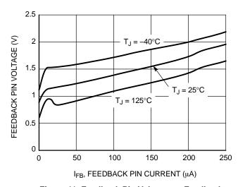
Figure 11. Feedback Pin Voltage vs. Feedback Current
