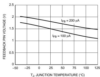
Figure 10. Feedback Pin Voltage vs. Temperature
