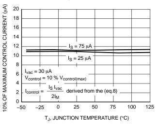
Figure 21. 10% of Maximum Control Current vs. Temperature
