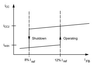
Figure 35. Undervoltage Protection
