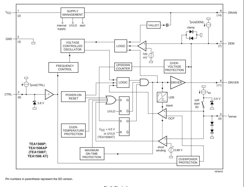
Fig.2 Block diagram.
