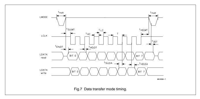
All transfers are bytewise, i.e. they are based on groups of 8 bits. Data will be stored in the TDA1315H after the eighth bit of each byte has been received. It is possible to read only the first byte of the channel status and of the TDA1315H status register.
