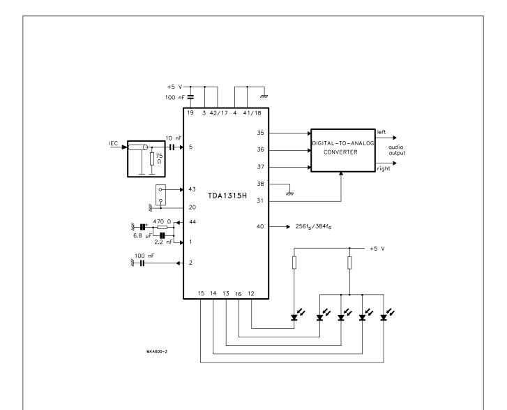
When in a system both IECIN1 and IECIN0 inputs are used, the signal that is applied to the IECIN0 input must be kept away from the IECIN1 input on the printed-circuit board. Steep slopes of the IECIN0 input can be seen by the sensitive adjacent IECIN1 input. An extra capacitance parallel to the 75  $\Omega$  resistor, close to the TDA1315H, can help reduce the crosstalk if required. A suitable value is 180 pF.
