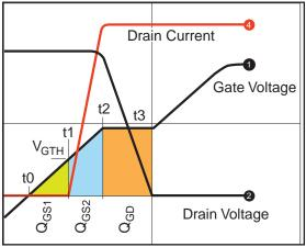
Figure 1: Typical MOSFET switching waveform
