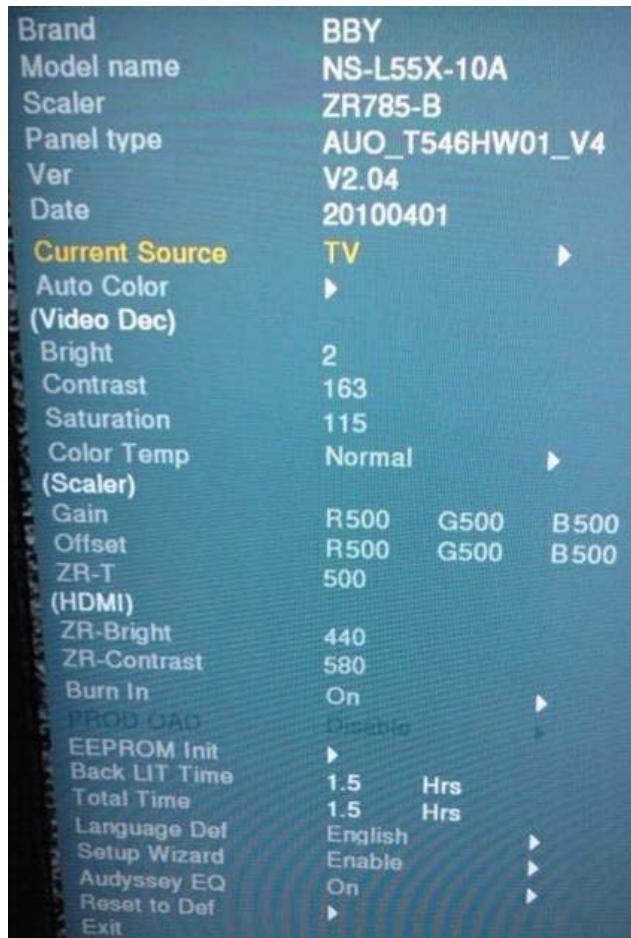
2. Change TV, press the item “Current Source” to Component mode and change signal to Timing314(Component 720p) and Pattern 122(SMPTE Bar), press the item “Auto Color”; Change TV, press the item “Current Source” to PC mode and change signal to PC TIMING 137(1024X768@60Hz) Pattern 147 (16 Grays), press the item “Auto Color”.
