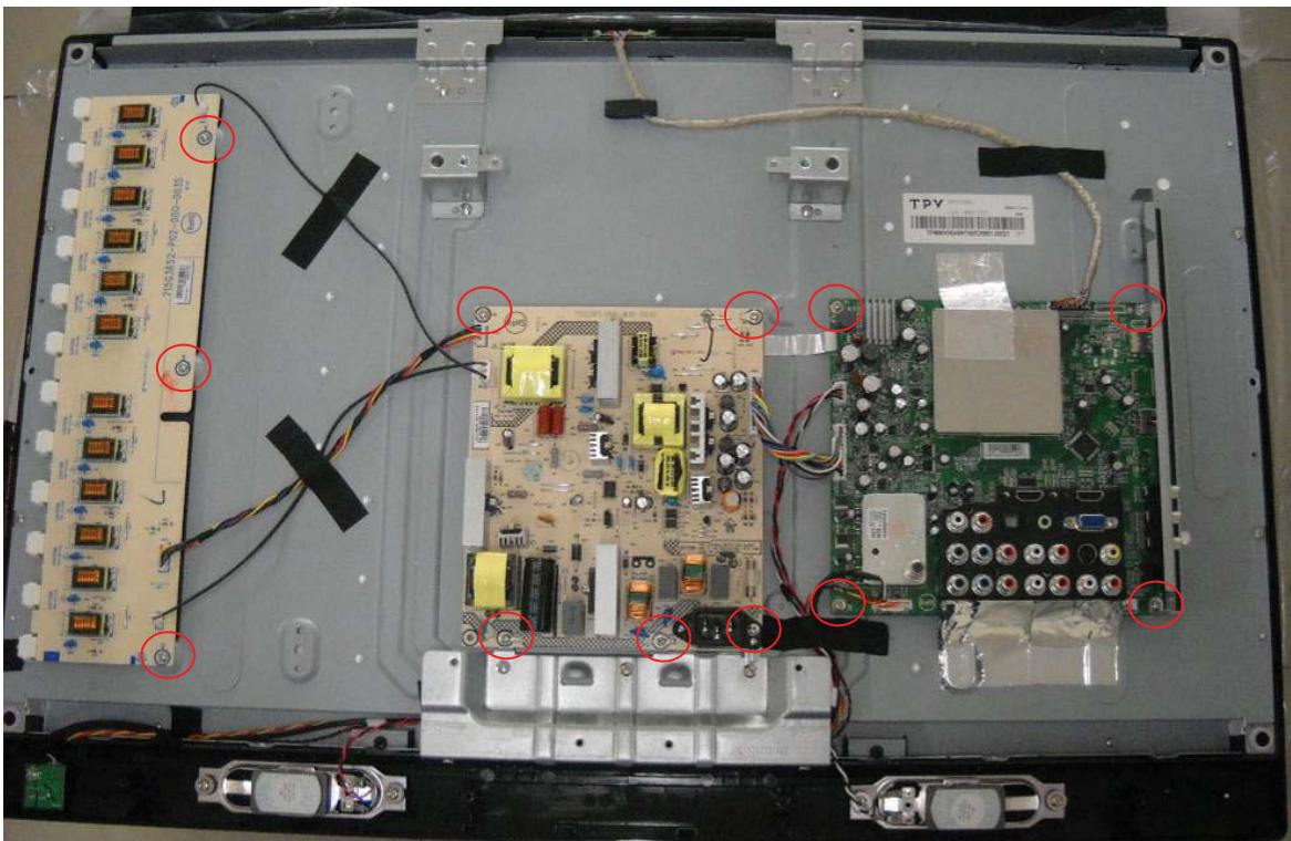
4. Remove the screws to remove bracket.
