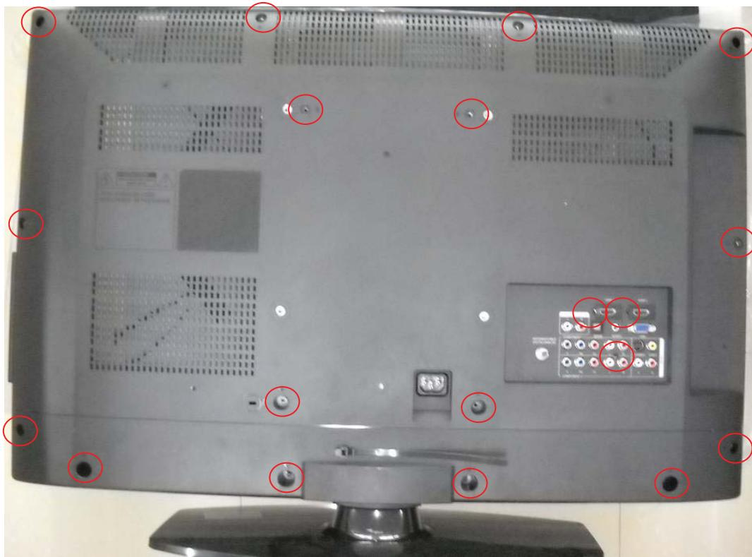
2. Remove the screws to remove stand base.
