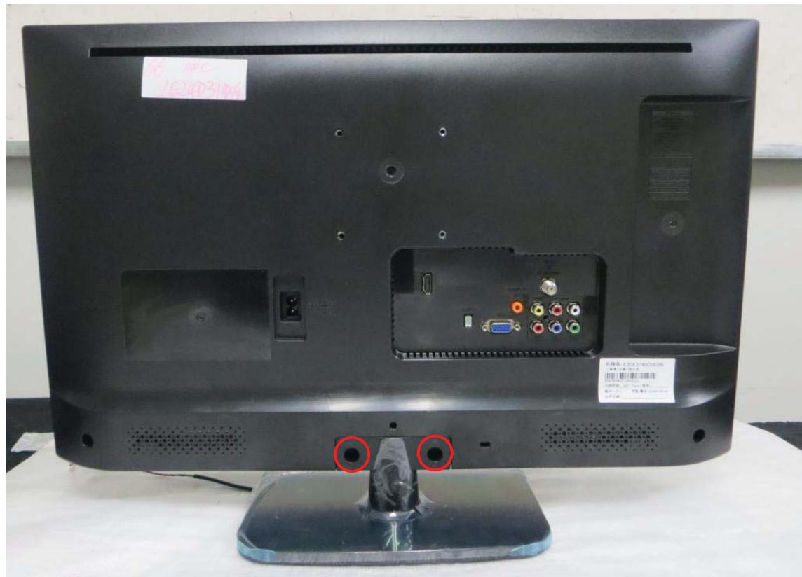
2. Remove the screws to remove REAR COVER.
