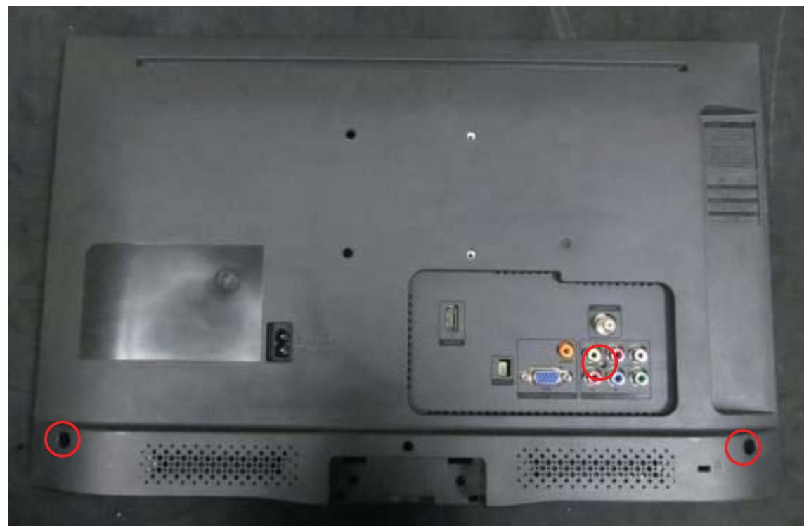
3. Disconnect the PINS marked in yellow .Remove the screws marked in red to remove MAIN BOARD, POWER BOARD and SPEAKERS.
