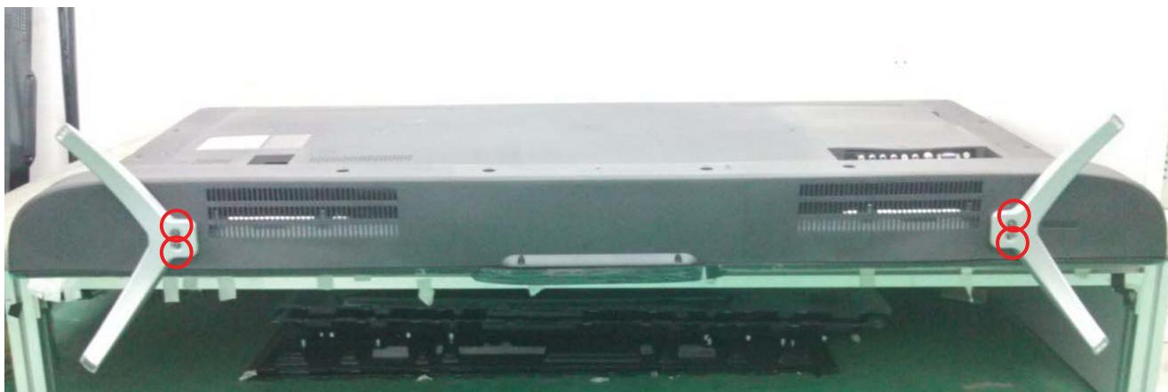
2. Remove the screws to remove REAR COVER.
