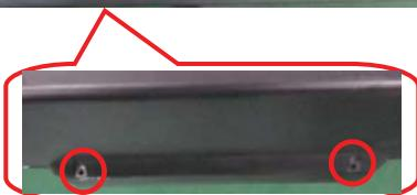
3. Disconnect the PINS marked in yellow. Remove the screws marked in red to remove MAIN BOARD,POWER BOARD,CONVERTER BOARD, BKT\_IO,SPEAKER.
