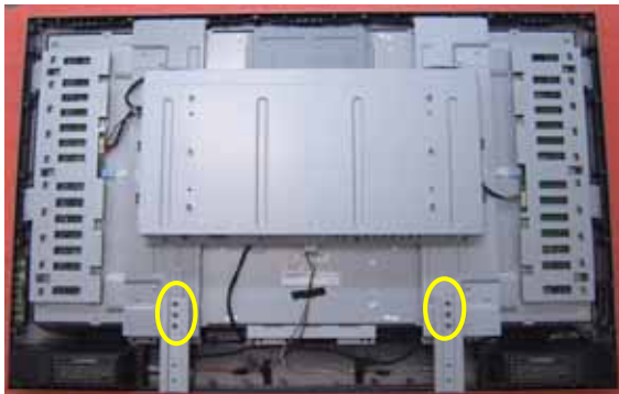
3. Remove 10pcs screws from rear cover and take off stand cover.
