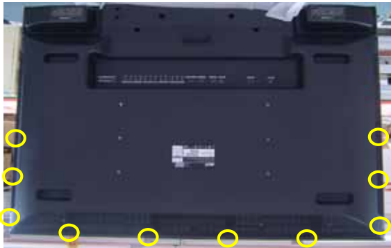
3. Remove 10pcs screws from rear cover and take off stand cover.
