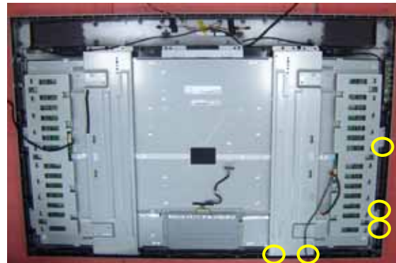
19. Remove 4pcs GND screws from P/B, M/B, IR/B and BTN, then take off it.
