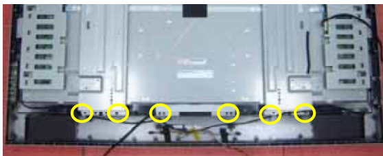
18. Remove 7pcs screws from M/B and P/B, then take off them.
