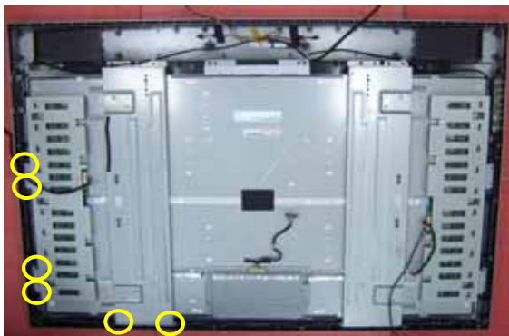
22. Remove 6pcs screws from panel, then separate panel and bezel.
