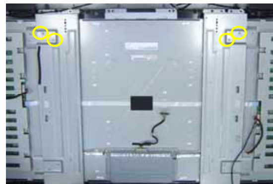
23. Remove 4pcs screws from EMI GASKET DOWN.
