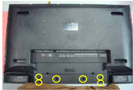
2. Remove 6pcs screw from base and stand cover.
