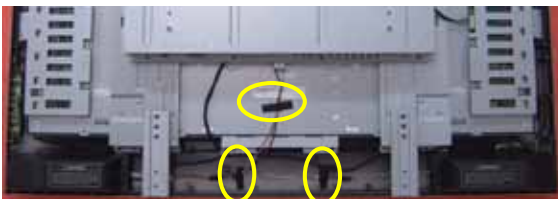
7. Remove 2pcs screws from HDMI joint and tear off the tapes.
