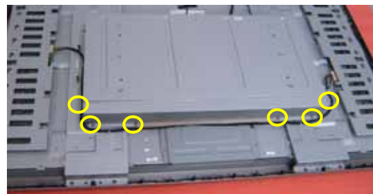
6. Remove 2pcs IO NUT from VGA joint and 7pcs screws from IO/B joint.
