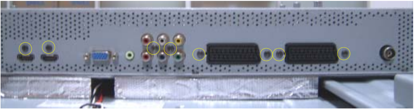
5. Release 6pcs screws from HDMI and IO joint.
