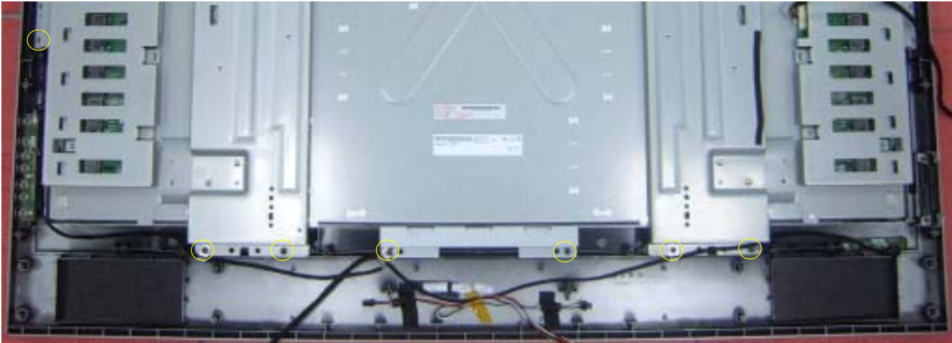
14. Release 7pcs screws from panel brackets.
