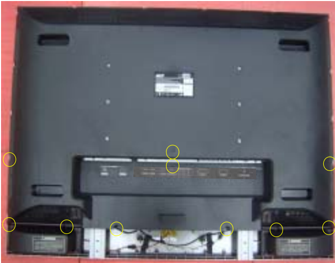
3. Release 10pcs screws from rear cover.
