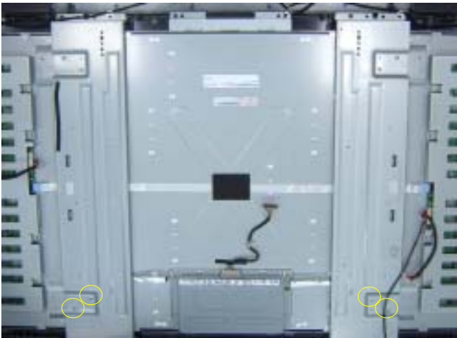
17. Release 4pcs screws from top panel brackets.
