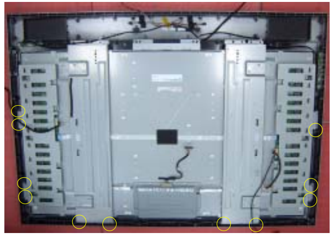
16. Release 11pcs screws from bezel and brackets.
