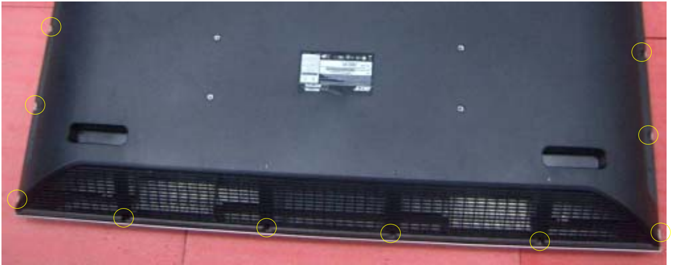
2. Release 10pcs screws from rear cover.
