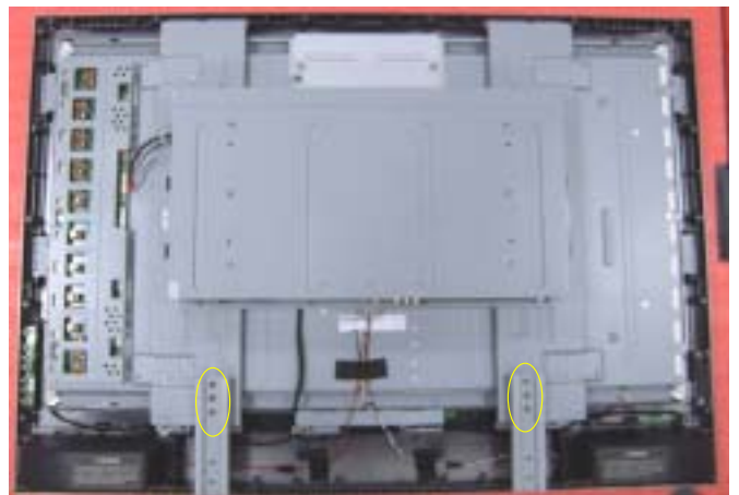
4. Release 6pcs screws from stand brackets.
