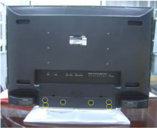
1. Release 6pcs screws from base and take off it.
