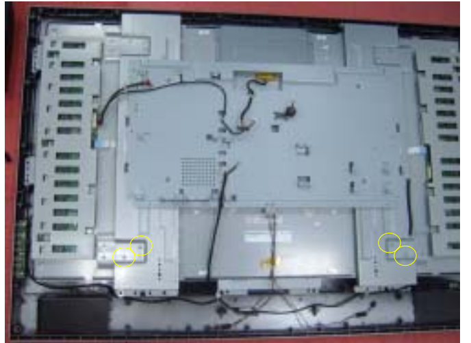
18. Release 4pcs screws from bottom panel brackets, then take off them.
